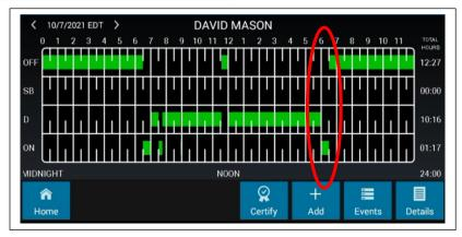
Using "Add" to edit we were able to enter the time we wanted the off-duty status to start (6:30pm) which left 30 minutes on-duty for the post trip. If we wanted to edit the entire status we would use the "Events" tab.
